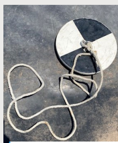
Figure 7. Standard Secchi disk design.
